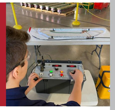
Abstract - Overvoltage tests, also known as high potential or "Hi-Pot", are used frequently to ensure the minimum dielectric strength of the insulation system. It is not a destructive test, nor does it degrade materials. These tests are carried out in whole or in part of the winding, to test the ground condition of the insulation of rotating electric machines.
