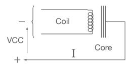
Figure 1. Basic setup of a DC Hi-Pot test.
